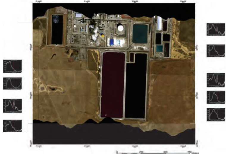
Georeferenced and radiometrically corrected microCASI airborne mosaic. Acquired March 19, 2016 over Nitrogen Production Facility, Carseland, AB. 50cm resolution: flight altitude 1000m, ground speed 75 knots. RGB Display bands: 714nm, 650nm, 550nm
