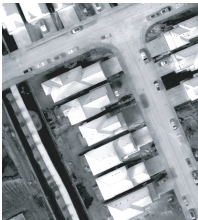
Radiometrically and georeferenced microTABI thermal image
