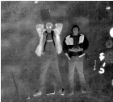
Detecting Acrylics/Nylon Using SWIR
