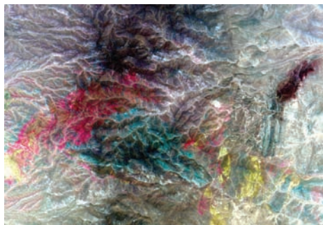
TASI-600 hyperspectral thermal night image, 70 cm, Yerington, Nevada (R: 9149nm G:10354nm B:11449nm)
